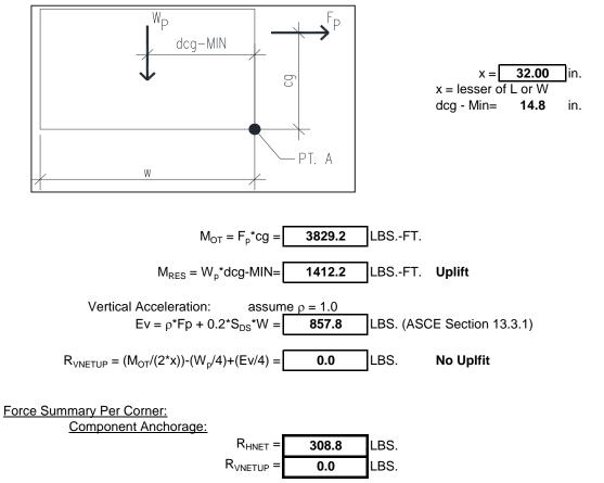
Anchors Embedded in Concrete or CMU:
